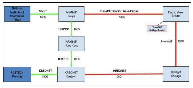
Figure 2: A diagram showing how the traffic was routed from the National Institute of Informatics (NII) to POSTECH, at first via the US, shown with a Red line, and then later staying in Asia, shown with a Green line.
