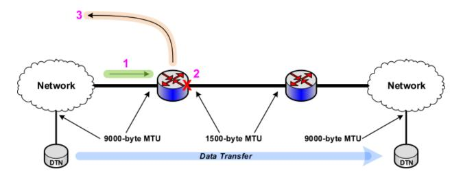
The diagram above illustrates the correct operation of PMTUD. The incoming jumbo packet (1) sent by the source DTN cannot be forwarded out the router's standard-frame interface, and because DF is set the packet is dropped (2). The router then sends an ICMP unreachable message (3) to the source address (in this case, the address of the sending DTN).
